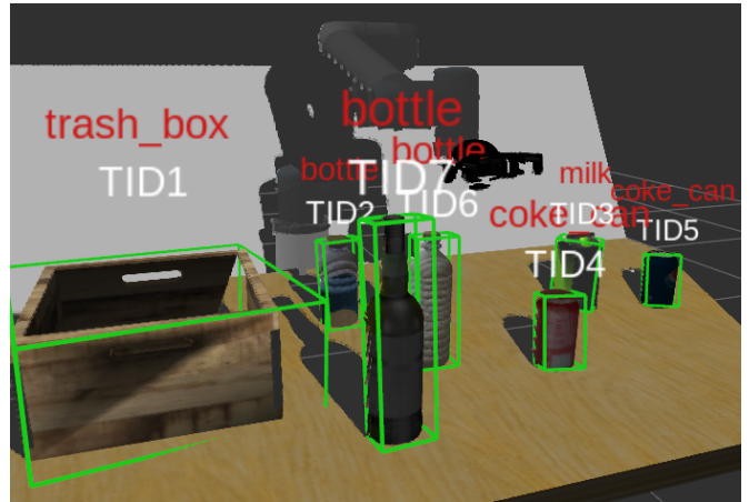
d) The RViz visualization of the recognized categories for the second robotic demonstration.
